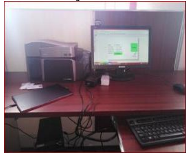
Card Printer: For printing chip based smart cards for registered users of the library
