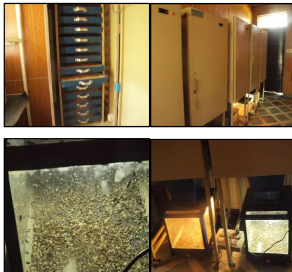
(Clock wise): Corcyra rearing machine; door opened to show sliding racks; adult Corcyra trapping device, trapped adult Corcyra
